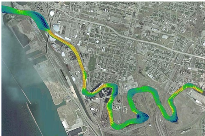
Using a suite of models, LimnoTech developed remedy footprints and sediment volume estimates.
